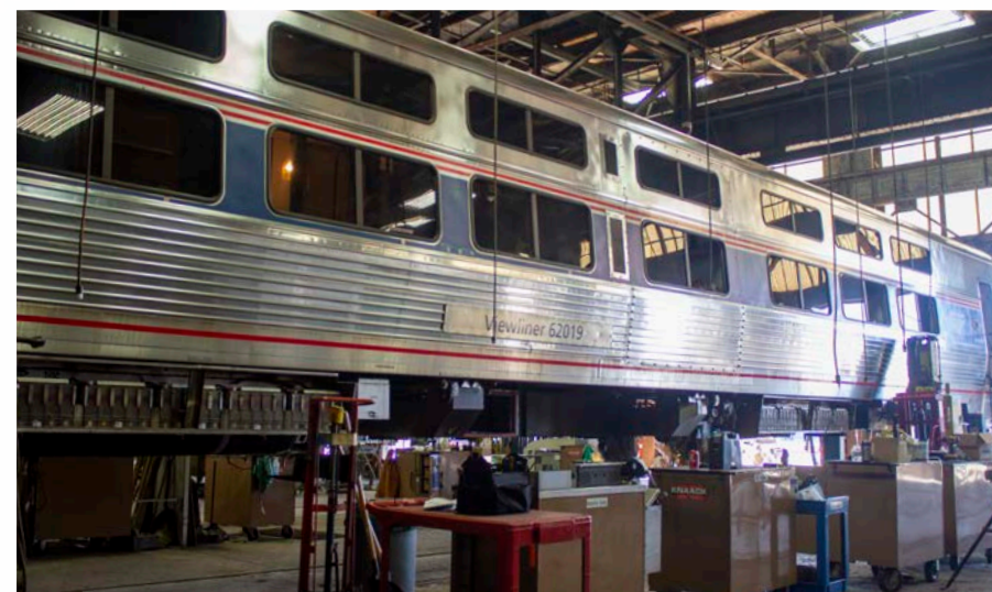
A 21-year-old Viewliner I sleeping car gets a full overhaul at Beech Grove, Ind., on Aug. 29, 2016. Amtrak needs a significant increase in shop forces at Beech Grove and elsewhere to get cars back in service and producing revenue. Bob Johnston
